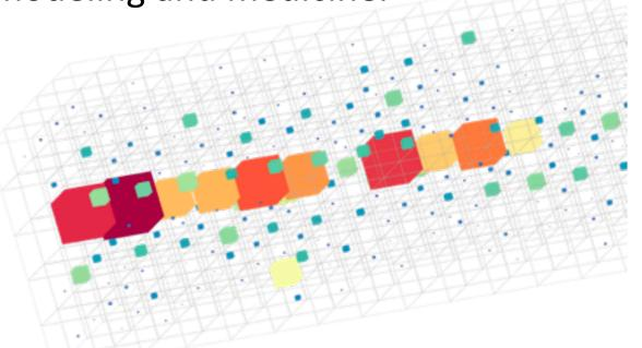
Single particle energy deposits in the Linear Collider Detector calorimeters generated by a GAN
