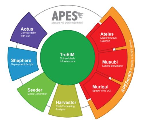
APES is a massively parallel CFD framework, which provides pre- and post-processing tools. It includes different solvers and allows the coupling of them using the integrated coupling approach APESmate.
