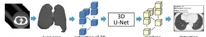
Fig. 6 Flowchart of automated detection of lung nodule in chest CT using 3D U-Net.
