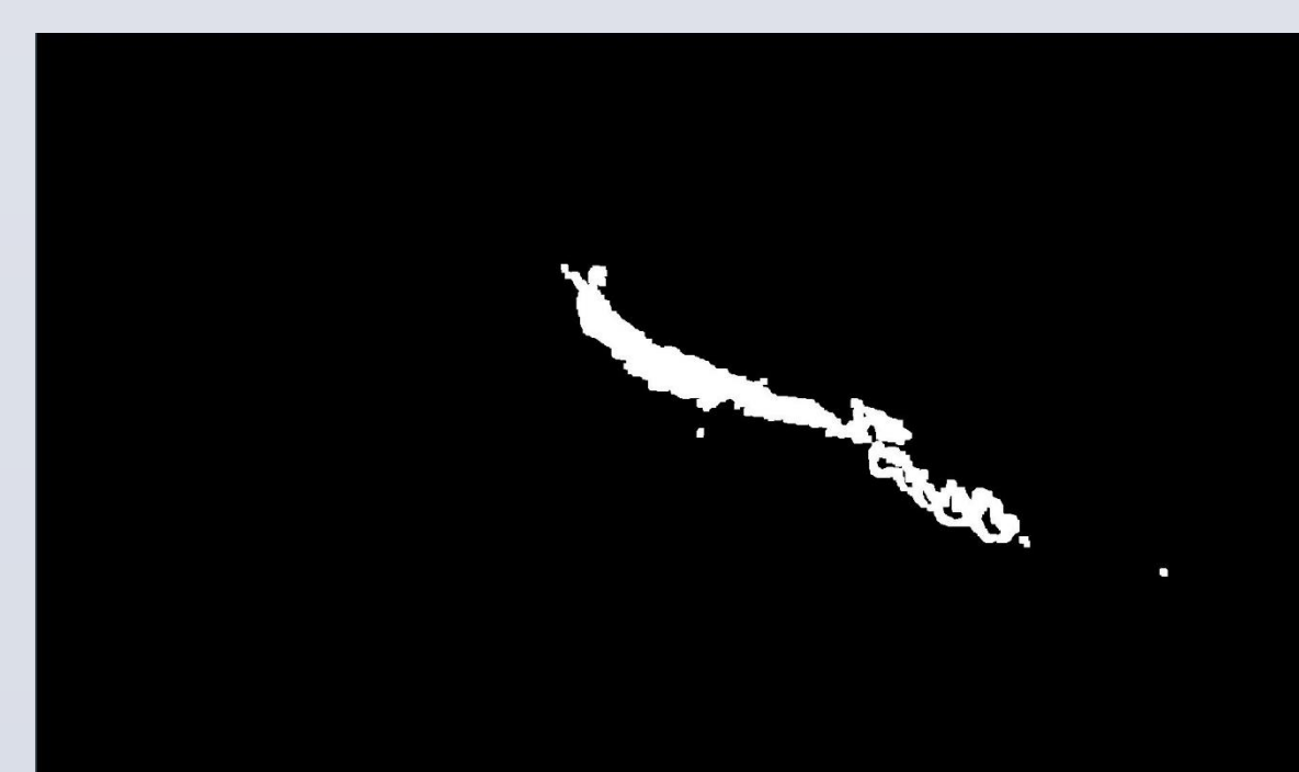
Figure 5. Shows a Threshold frame after dilate and erode
