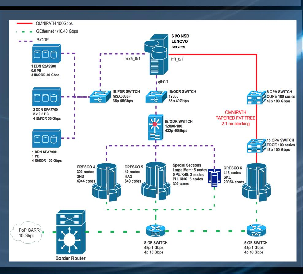
have 2 tier 2:1 no-blocking tapered fat-tree topology. The consumption of electrical power during massive computing workloads amounts to 190kW.
