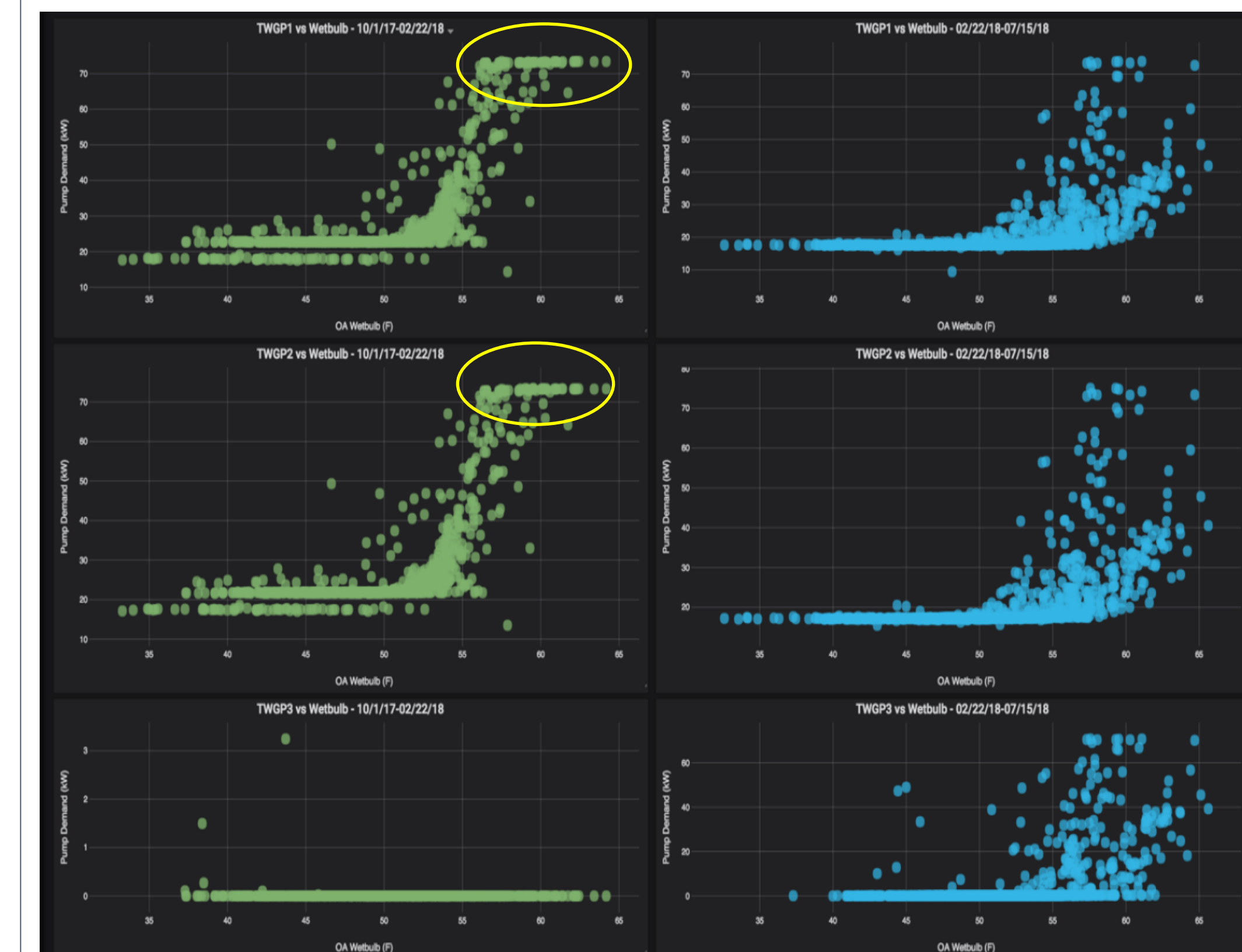
Figure 7, Benefits of HX Retrofit on Tower Water Pump Demand. The baseline draw for Pumps 1 & 2 is ~20kW while it is 0kW for Pump 3. Pumps 1 & 2 cannot be turned off because they are open enclosure systems. If turned off, outside elements (moisture, smoke particulates, etc.) have the chance to accumulate and can ultimately corrode the equipment. In contrast, Pump 3 is a closed enclosure system, thus it can selectively turn on only when it is needed.
