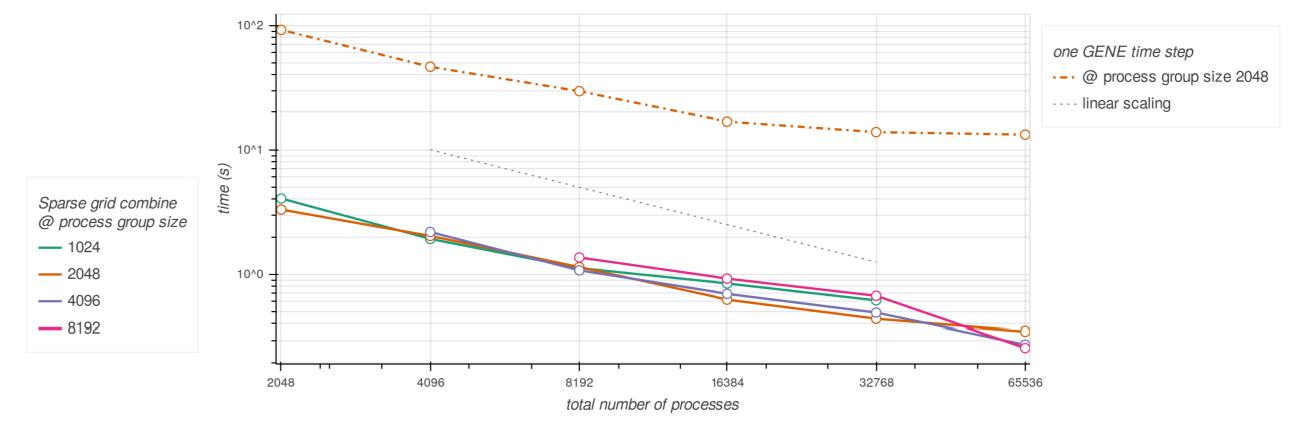
The combination technique overhead scales at a level negligible to the GENE set-up
